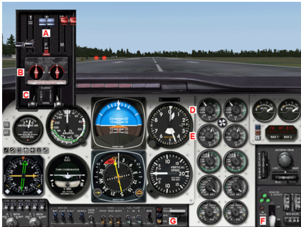
Figure 1-1 A-Propeller Controls B-Fuel Selector C-Cowl Flaps D-Manifold Pressure E-Propeller RPM F-Landing Gear G-Flaps
